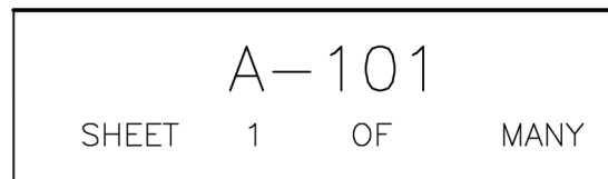
Figure 02.10 Sheet identification block.
