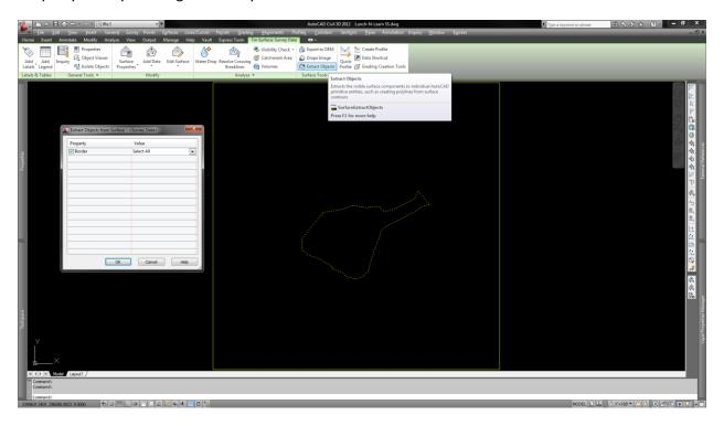
Create a **stepped offset** of about 20'± (more or less, depending on how wide the blend zone needs to be). This is dependent upon the quality of the LiDAR. WV is notoriously bad and sometimes needs a wider zone for the blend.
