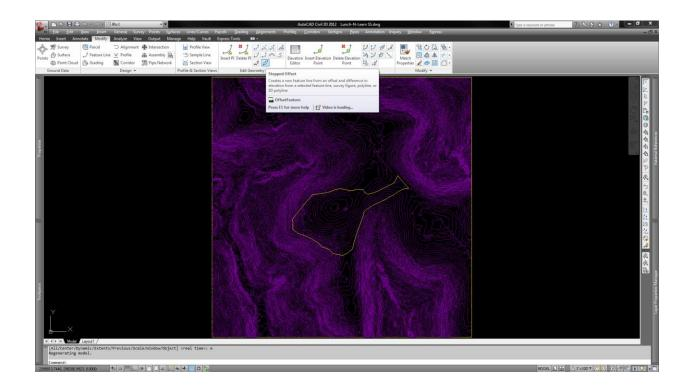
Use the ribbon button to assign elevations from surface EG (your LiDAR or target surface).
